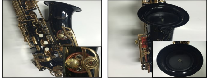
Figure 3. Installed saxophone interface
